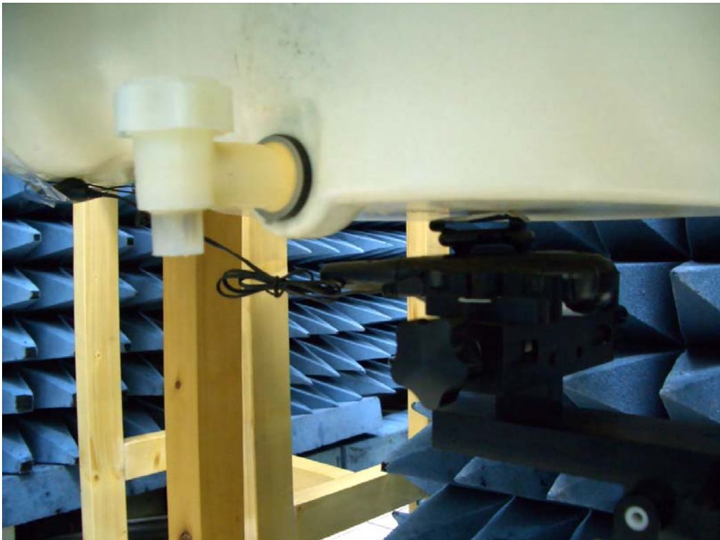
Figure15. SAR Test Setup w/Belt Clip
