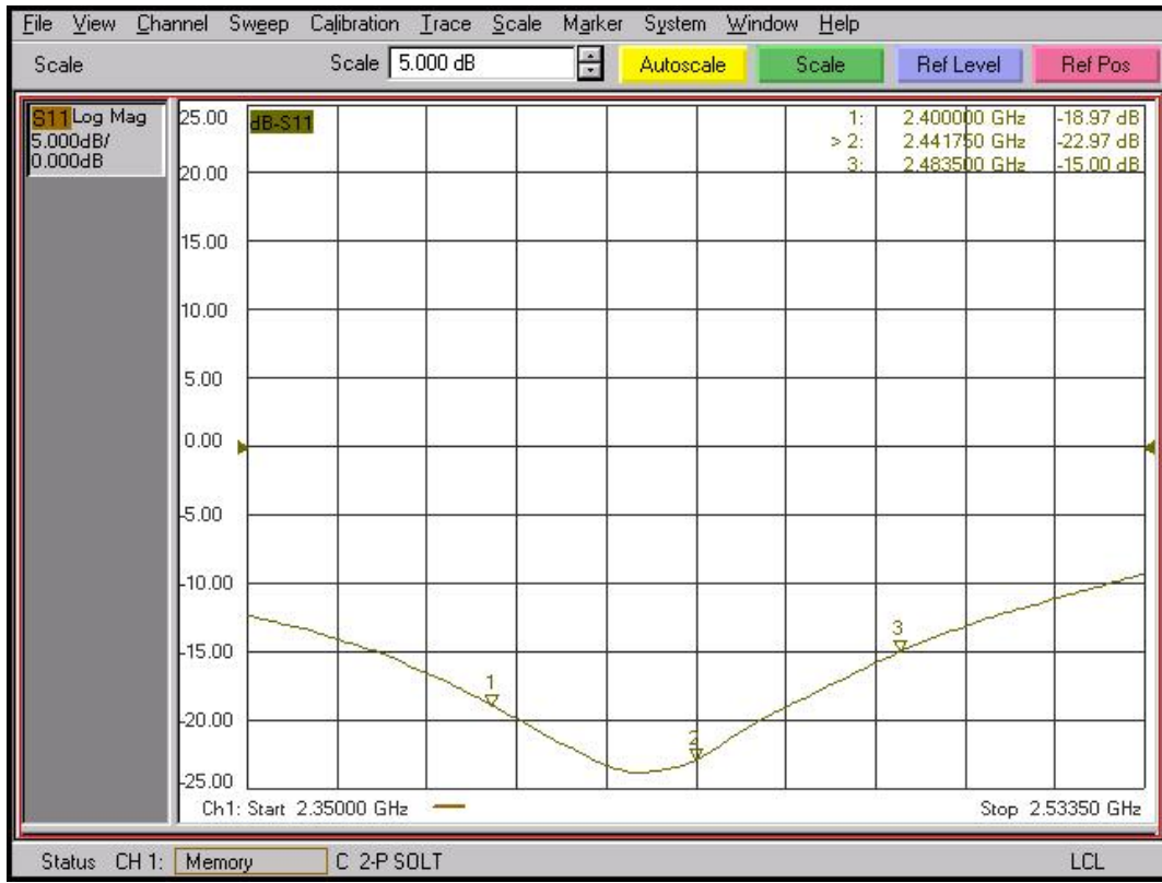
Fig 2. V.S.W.R (Agilent E8357A 300KHz~6GHz PNA Series Network Analyzer)
