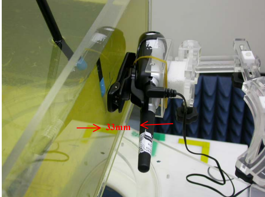
Figure 5: For body, EUT rear with belt-clip and microphone to phantom, 0 mm separation-Zoon In
