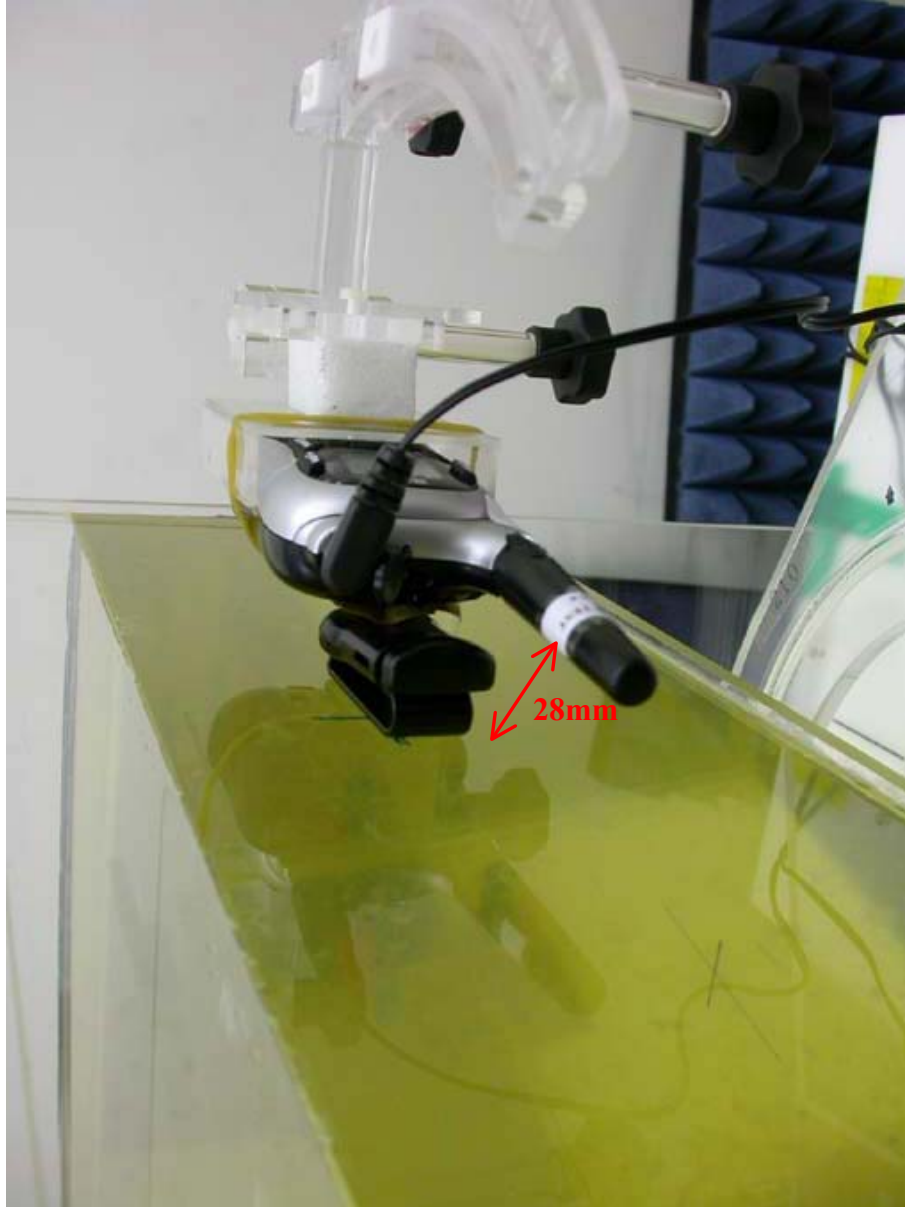
Figure 5: For body, EUT rear with belt-clip and microphone to phantom, 0 mm separation-Zoom In
