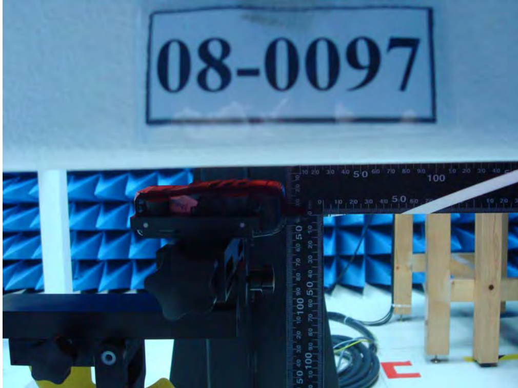
Figure 17. SAR Test Setup _ Face Position
