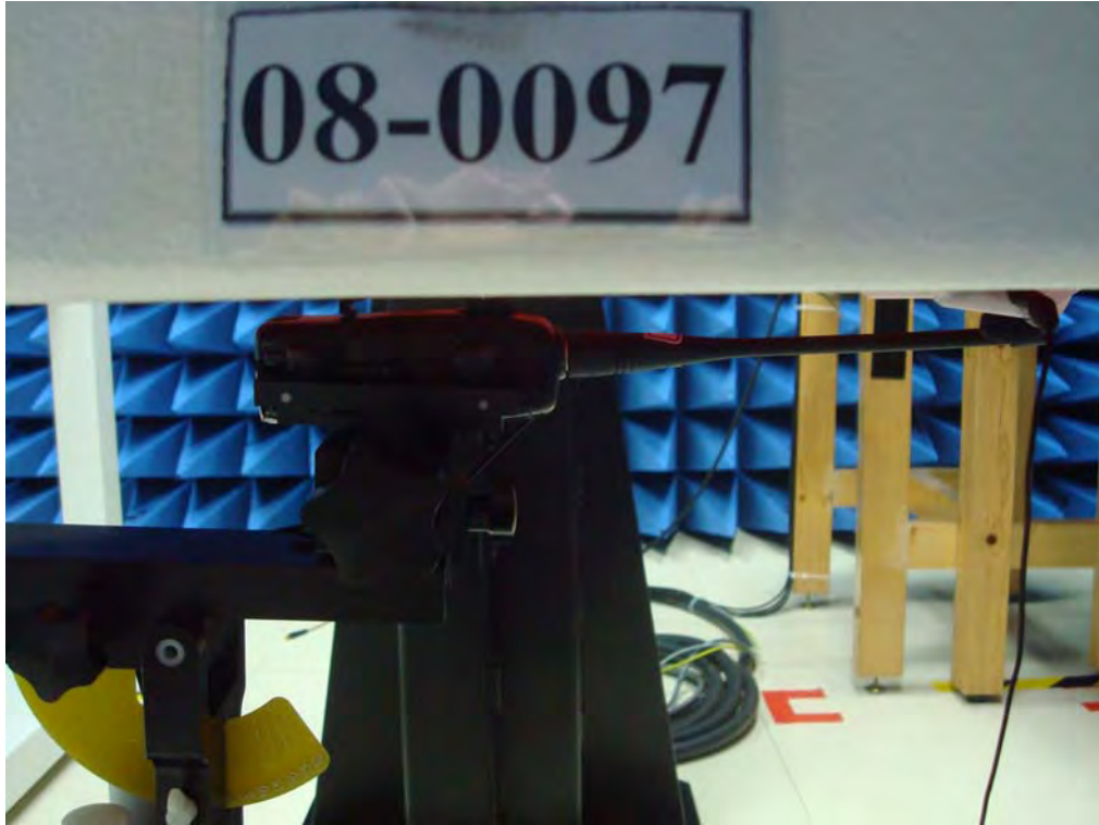
Figure 19. SAR Test Setup _ Body Position with Headset and Belt Clip
