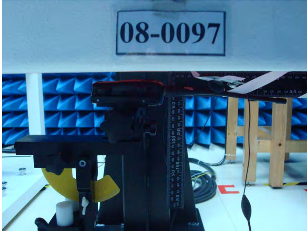
Figure 18. SAR Test Setup _ Body Position with Headset _ 15mm space
