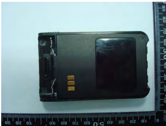
Figure 5. Li-ion Battery ( 7.4V 1100mAh )
