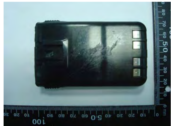
Figure 5. Li-ion Battery ( 7.4V 1100mAh )
