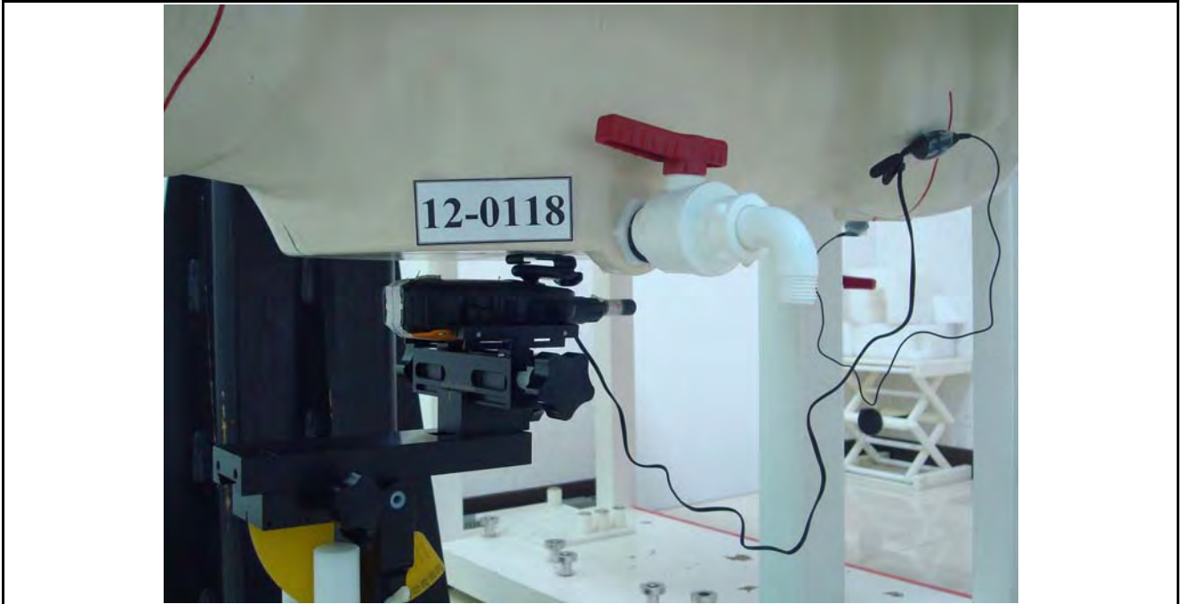
Figure 4. Body SAR Test Setup (Flat Section)
