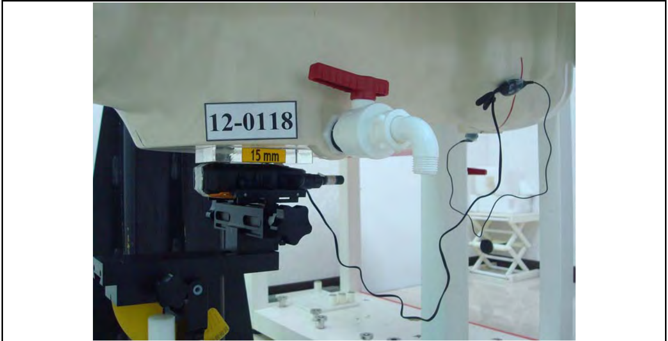
Figure 3. Body SAR Test Setup (Flat Section)
