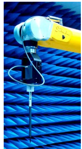
Figure 13. Probe setup on robot
