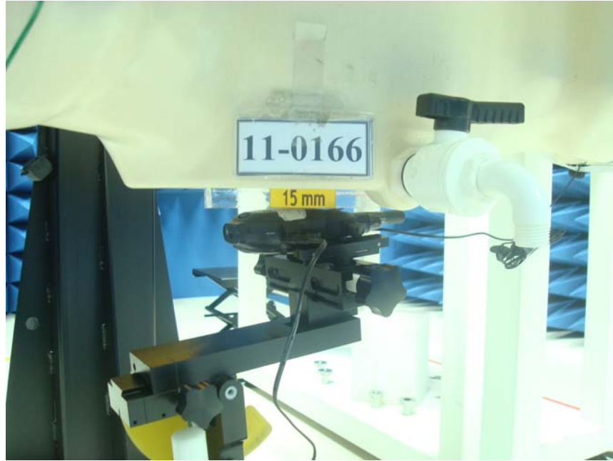
Figure 24. EUT (Charging by AC Adapter) link headset distance phantom 15mm (The Spacer was removed during SAR testing)
