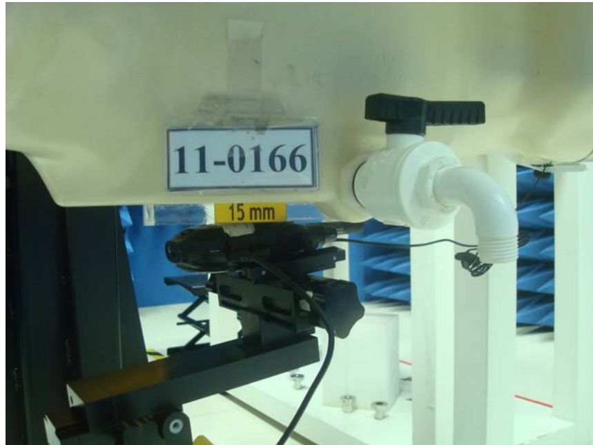
Figure 23. EUT (Charging by USB cable via computer) link headset distance phantom 15mm (The Spacer was removed during SAR testing)
