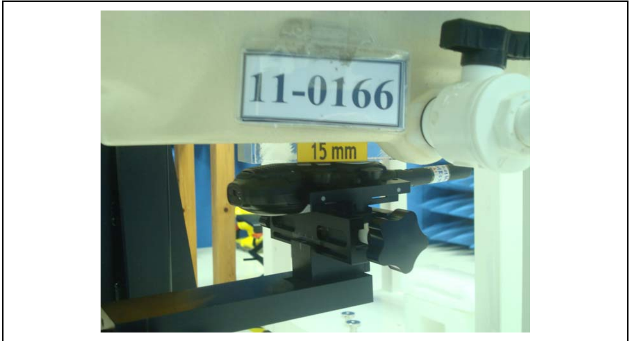
Figure 19. EUT front side distance phantom 15mm (The Spacer was removed during SAR testing)
