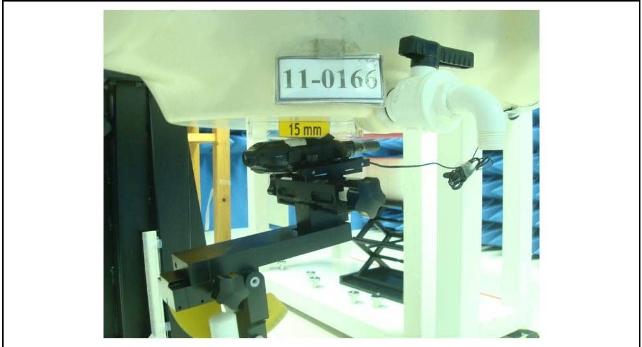
Figure 22. EUT link headset distance phantom 15mm (The Spacer was removed during SAR testing)
