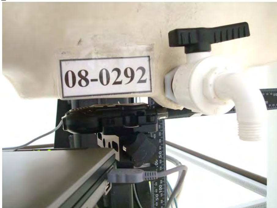
Figure 20. EUT Face to Phantom 15 mm spacing (Charging by USB Cable via computer)
