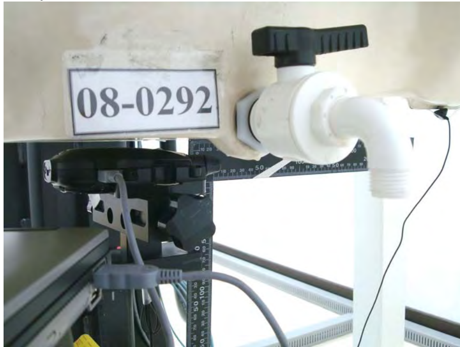
Figure 23. EUT with Headset to Phantom 15 mm spacing (Charging by USB Cable via computer)
