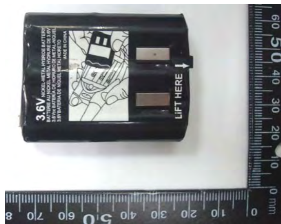
Figure 5. Ni-MH Battery ( 3.6V 650mAh )
