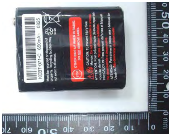
Figure 5. Ni-MH Battery ( 3.6V 650mAh )
