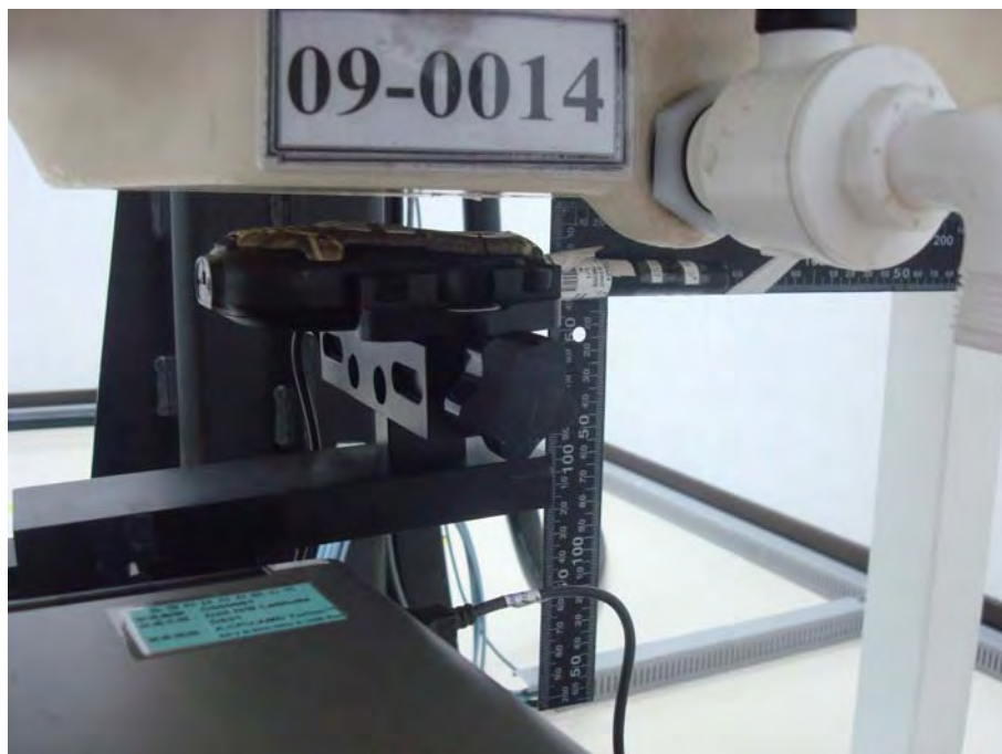
Figure 19.EUT Face to Phantom 15 mm spacing (Charging by USB Cable via computer)
