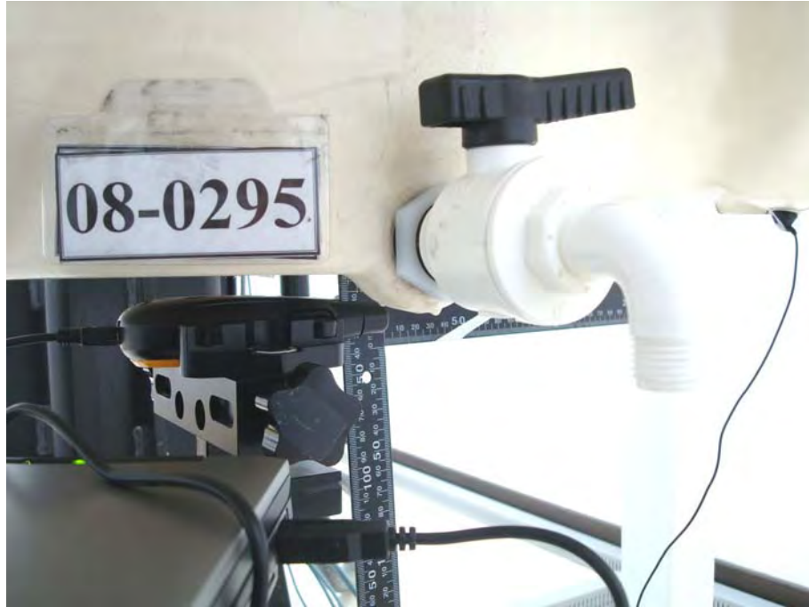
Figure 21. EUT with Headset to Phantom 15 mm spacing (Charging by USB Cable via computer)
