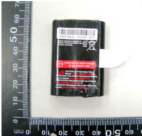
Figure 5. Ni-MH Battery ( 3.6V 700mAh )
