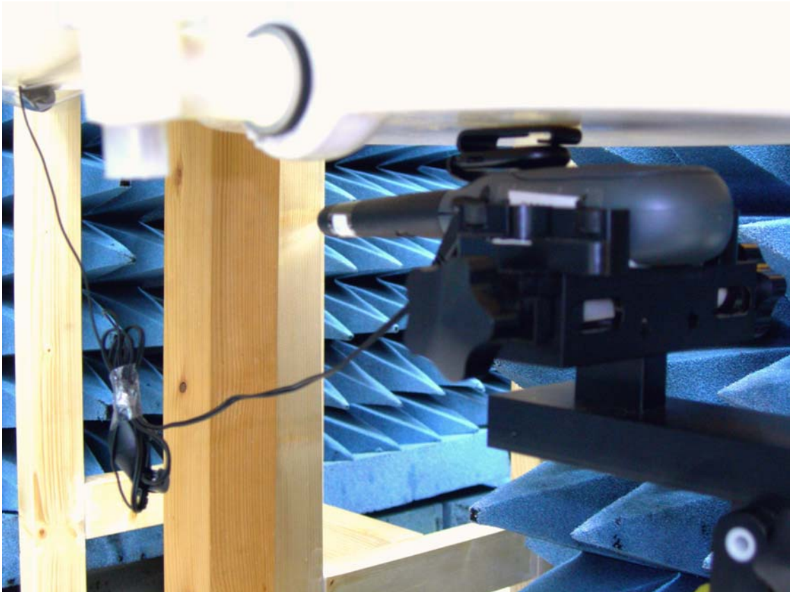
Figure16. SAR Test Setup w/Belt Clip
