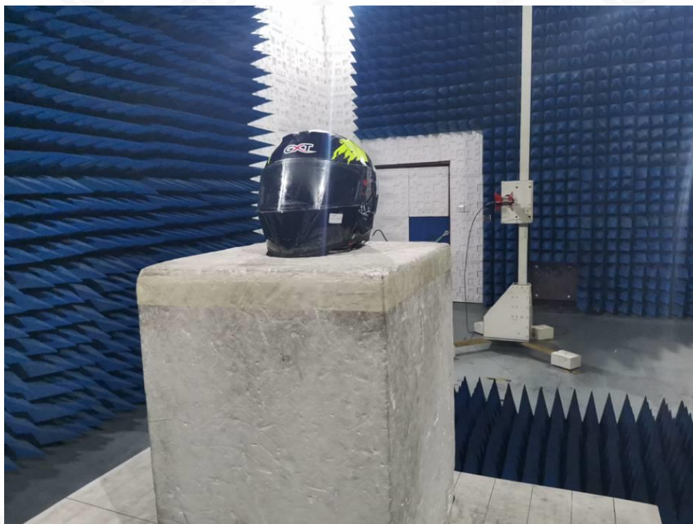
RADIATED EMISSION TEST SETUP ABOVE 1GHZ
