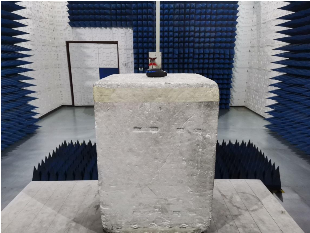
RADIATED EMISSION TEST SETUP ABOVE 1GHz
