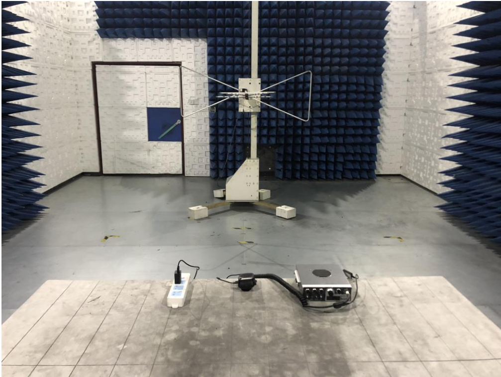
RADIATED EMISSION TEST SETUP ABOVE 1GHZ
