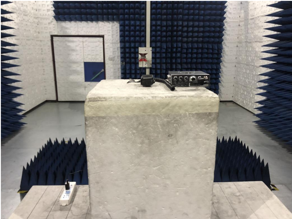
RADIATED EMISSION TEST SETUP ABOVE 1GHZ
