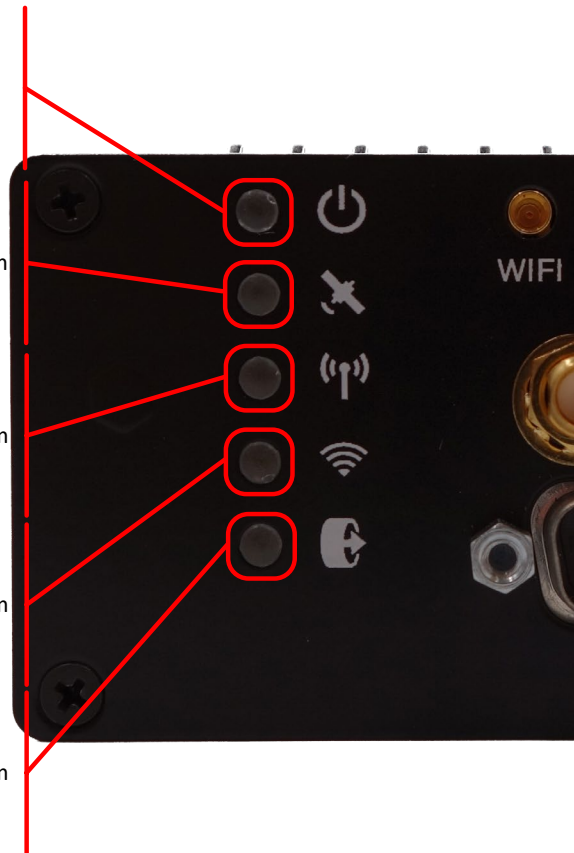
Figure 17 - IDU Status LEDs
