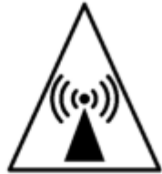
NON-IONIZING RADIATION HAZARD
