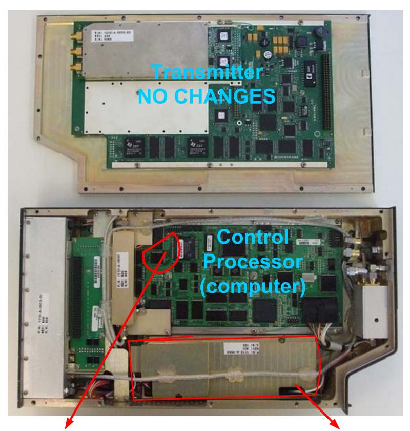
Memory for processor has been added in this section of the Control Processor (computer)
