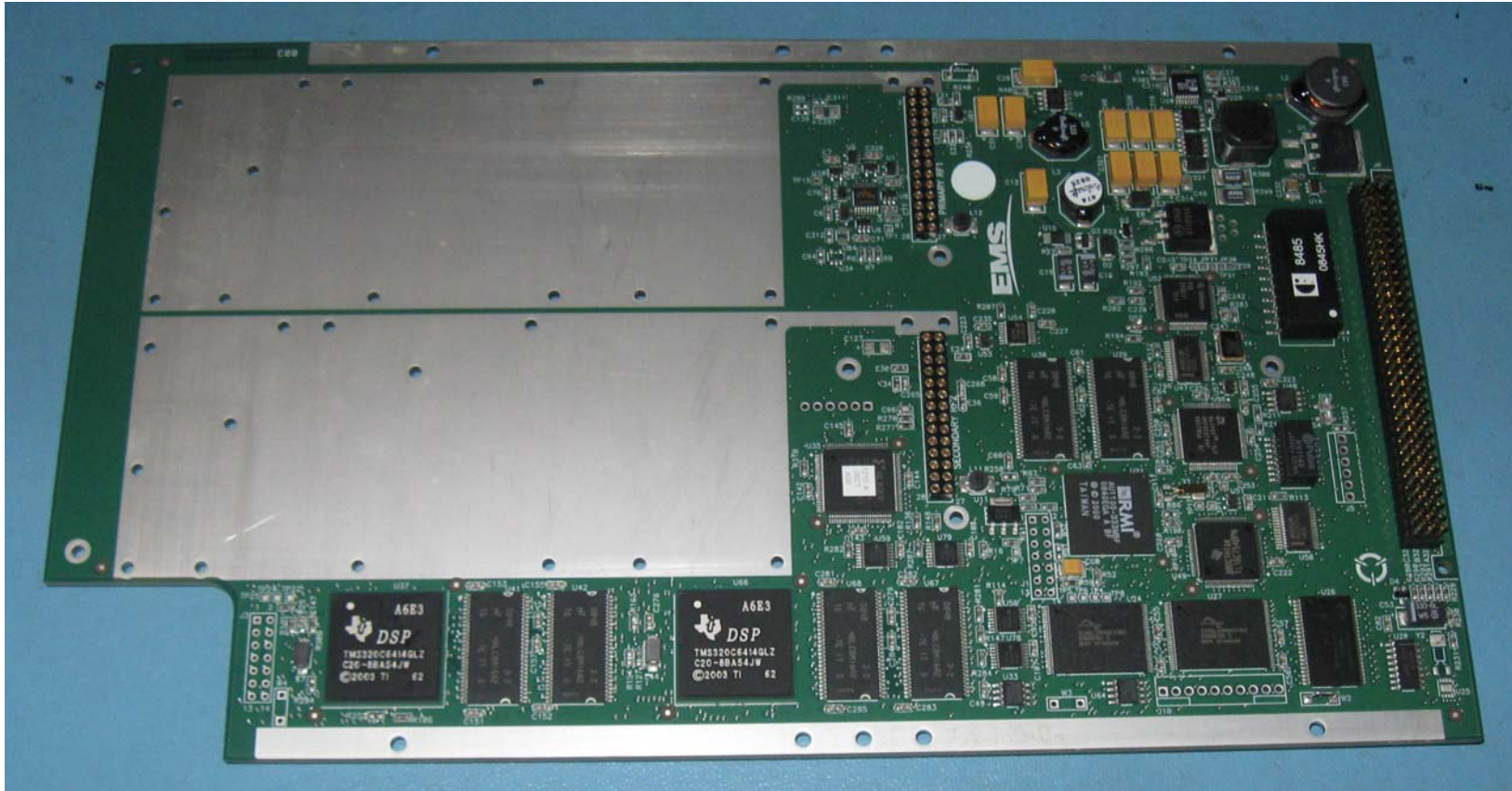
Figure 5: HST Digital Module 1210-A-0002-03 Top (Part of the HST BGAN 1 Channel Card)
