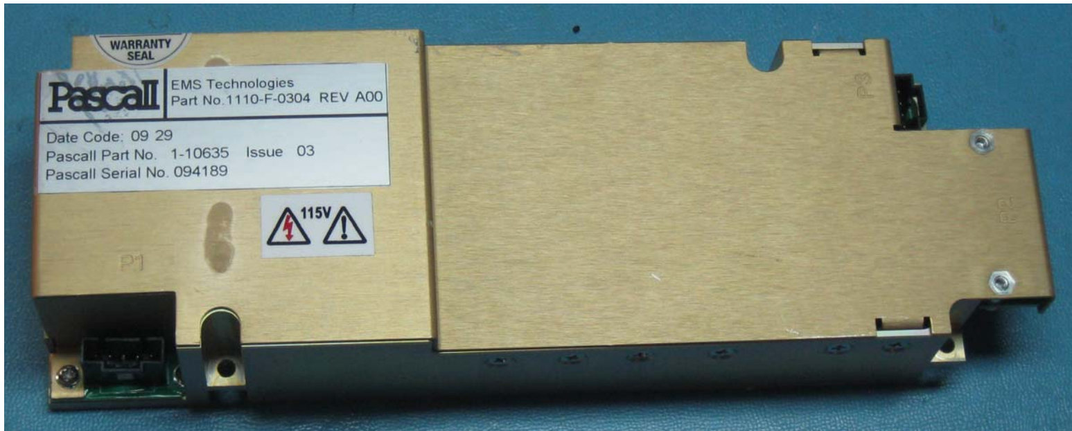
Figure 12: 1110-F-0304 HST Power Supply Top
