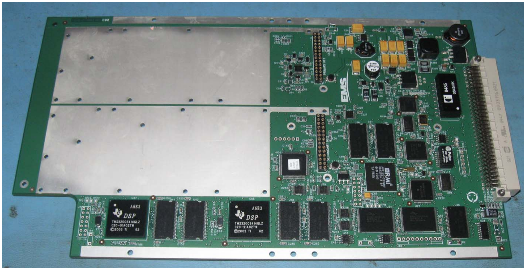
Figure 9: 1210-A-0002-01 HSD Digital Module Top (Part of the BGAN 2 Channel Card)
