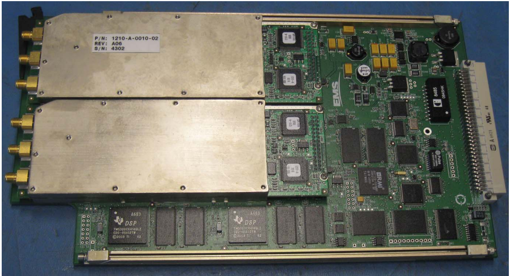
Figure 7: 1210-A-0010-02 BGAN 2 Channel Card Top
