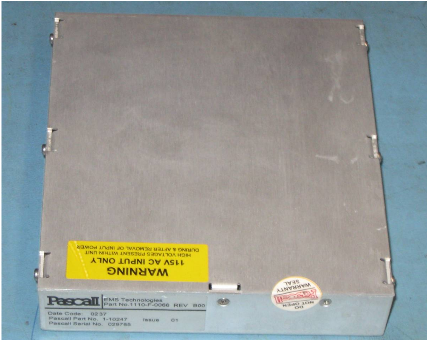
Figure 12: 1110-F-0066 Power Supply Top
