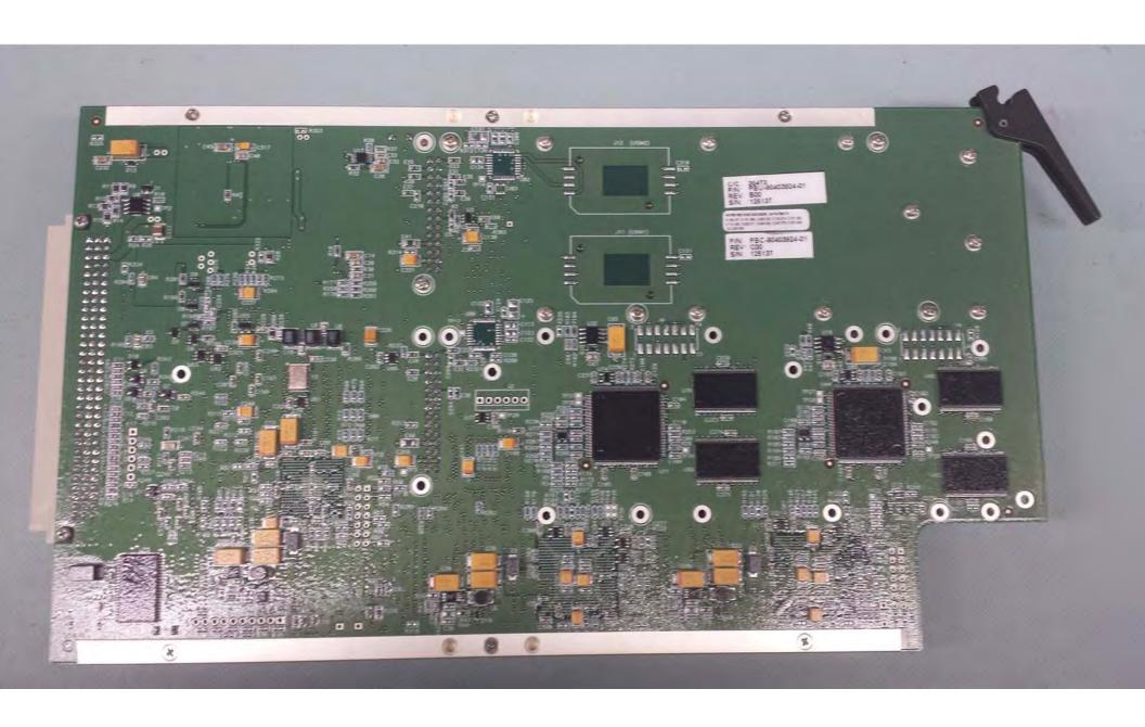
BGAN RF Card - Bottom (removed from piggyback, cover off)
