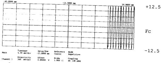
Trigger mode : Edge On Positive Edge Of Chan2 Trigger Level Chan2 = -412.500 mV (noise reject ON) Holdoff = 40.000 ns
