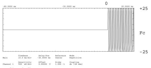
Trigger mode: Edge On Positive Edge Of Chan2 Trigger Level Chan2 = -481.250 mV (noise reject ON) Holdoff = 40.000 ns
