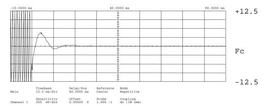
Trigger mode : Edge On Negative Edge Of Chan2 Trigger Level Chan2 = -4.000 mV (noise reject ON) Holdoff = 40.000 ns
