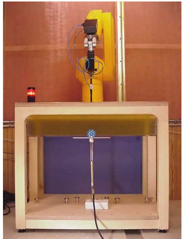
DASY3 SAR Measurement System with small planar phantom DASY3 SAR Measurement System with validation phantom
