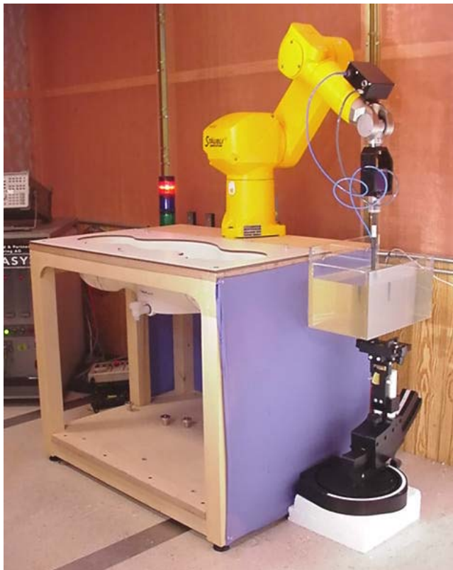
DASY3 SAR Measurement System with small planar phantom DASY3 SAR Measurement System with validation phantom
