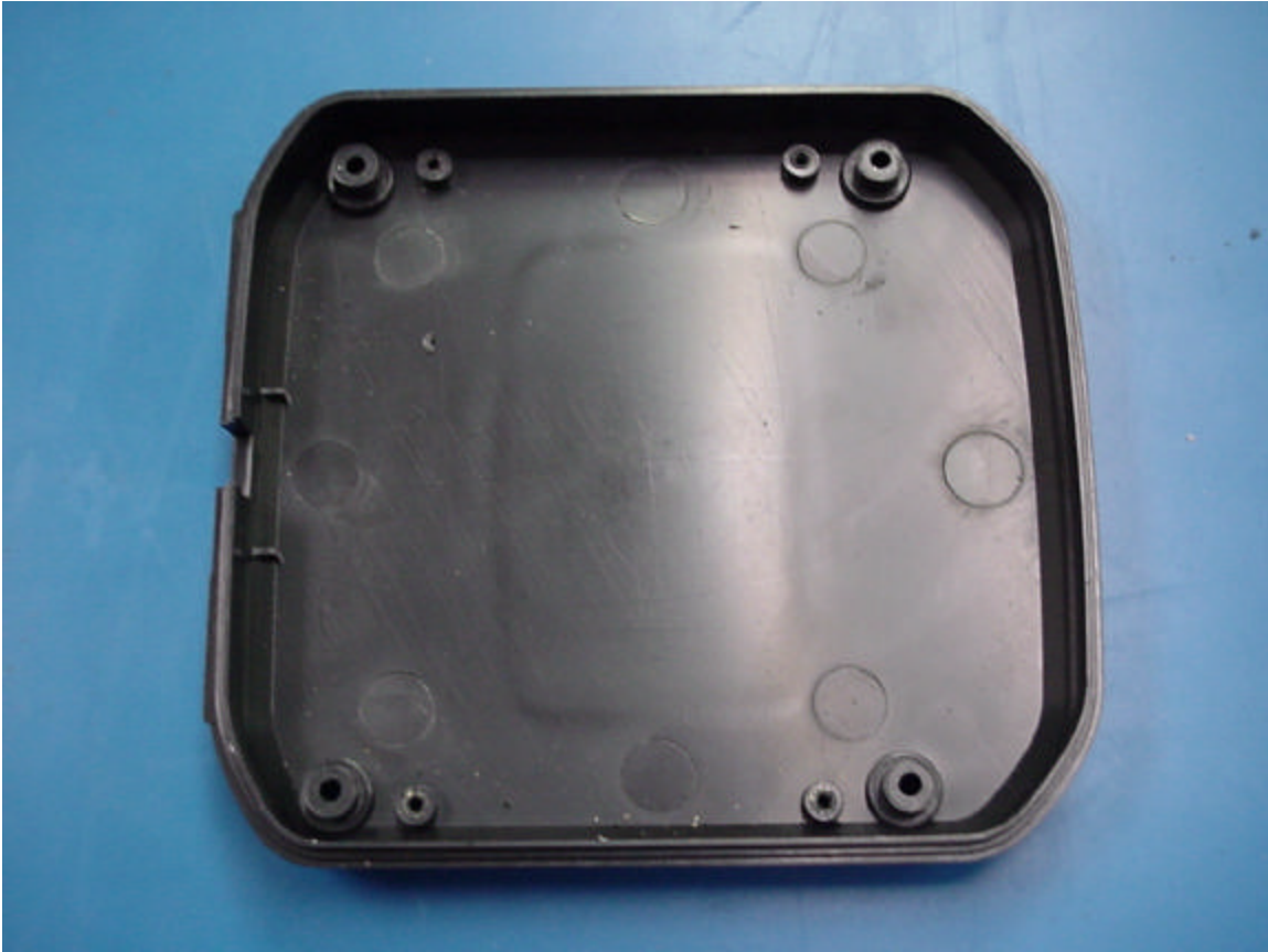
Inside Bottom of Battery Charger Chassis
