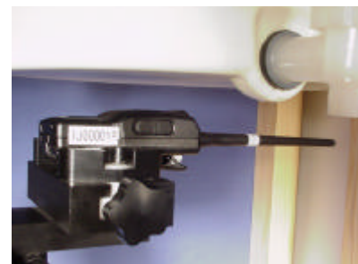
Face-held SAR Test Setup 2.5cm Separation Distance
