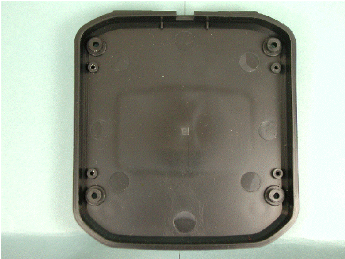
Inside bottom of battery charger chassis
