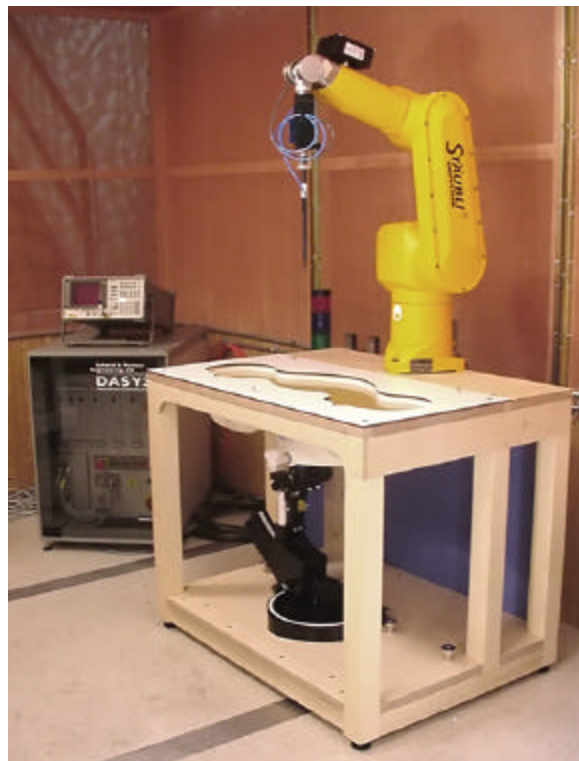
DASY3 SAR Measurement System with SAM phantom
