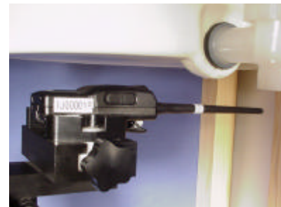
Face-held SAR Test Setup 2.5cm Separation Distance
