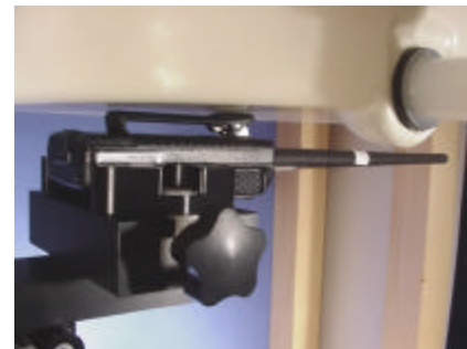
Body-worn SAR Test Setup with 1.4cm Belt-Clip
