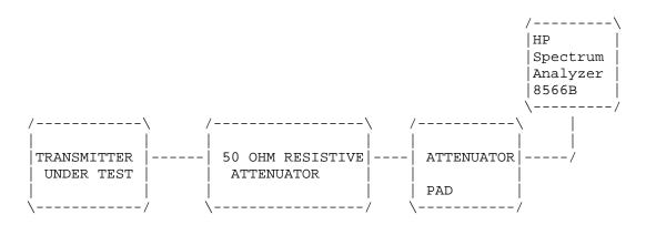
NAME OF TEST: SPURIOUS EMISSIONS AT ANTENNA TERMINALS
