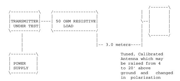
Equipment placed 4' above ground on a rotatable platform.
