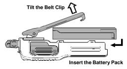
☐ To remove the battery, turn the radio off and remove any protective cases. Slide the **Battery Pack Latch** on the bottom of the radio toward the front panel while sliding the battery down about 1/2 inch. Then lift the battery out from the radio while unfolding the Belt Clip.
