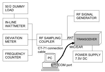
The transceiver must be programmed for use in the intended system before alignment is attempted. The RF parameters are loaded from the file during the alignment process. In order to facilitate alignment over the complete operating range of the equipment, it is recommended that the channel data in the transceiver be preset as per the chart below.
