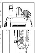
**MONITOR** button more than 2 seconds (or press the **MONITOR** button twice) to quiet the noise and resume normal (quiet) monitoring.
