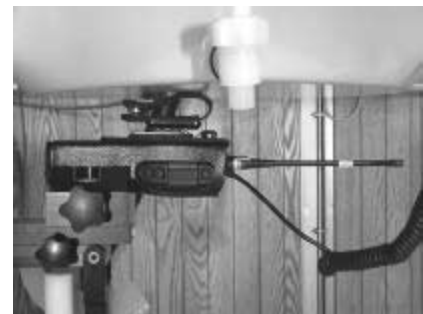
Body SAR Test Setup with Holster #2
