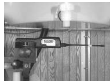
Face-held SAR Test Setup
