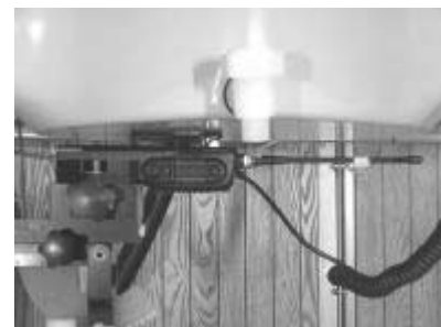
Body SAR Test Setup with Belt-Clip
