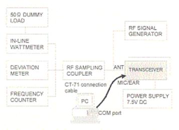
The transceiver must be programmed for use in the intended system before alignment is attempted. The RF parameters are loaded from the file during the alignment process.
