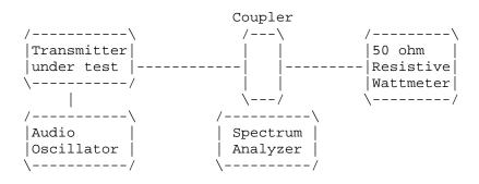
2.991 Spurious\_emissions\_at\_antenna\_terminals(conducted): Data on the following page shows the level of conducted spurious responses. The carrier was modulated 100% using a 2500Hz tone. The spectrum was scanned from 0.4 to at least the 10th harmonic of the fundamental. The measurements were made in accordance with standard TIA/EIA-603.
