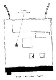
Setup the test equipment as shown for transceiver alignment, apply 13.6V DC power to the transceiver. Refer to the drawings above for Alignment Points.
