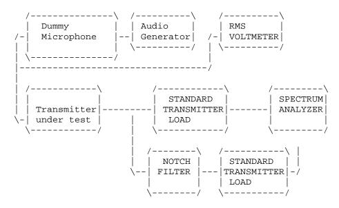
Method of Measuring Conducted Spurious Emissions
