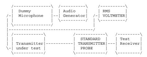
1. The test receiver audio bandwidth was <50Hz to >20,000Hz.
