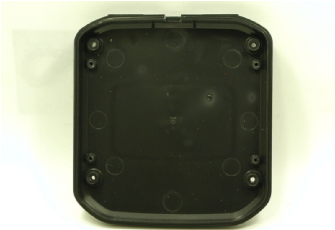
Inside bottom of battery charger chassis
