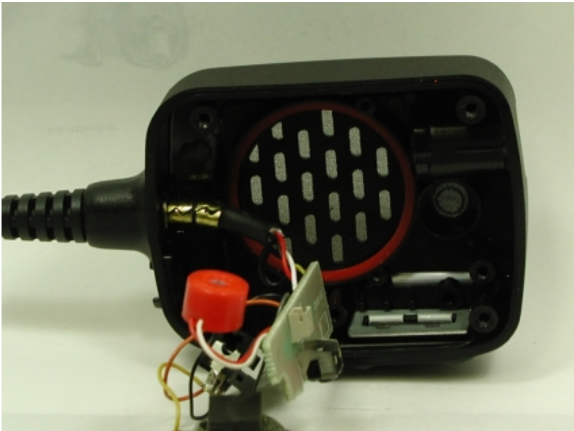
Inside of Back Microphone Chassis
