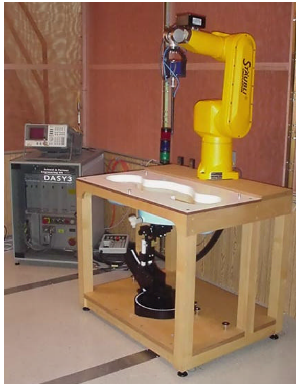
DASY3 SAR Measurement System
