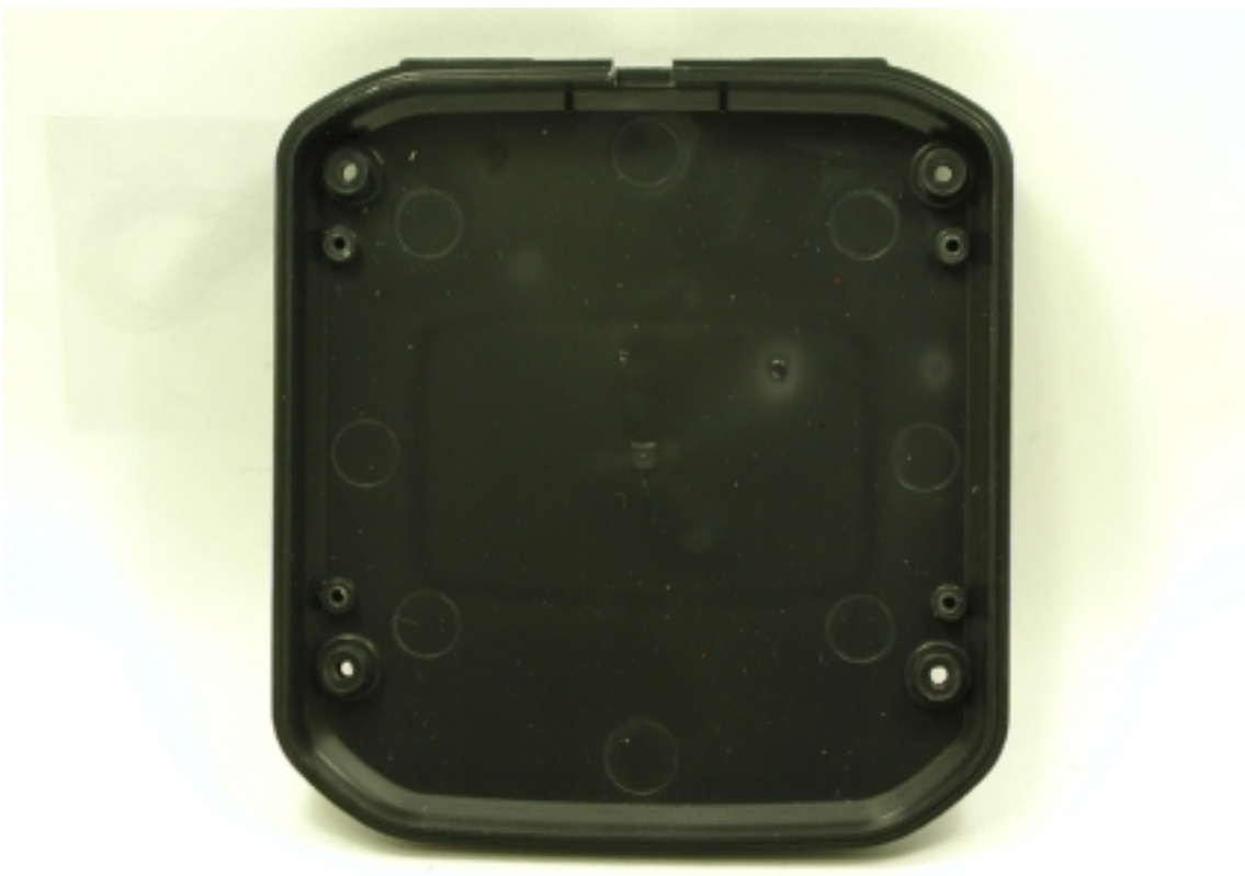
Inside bottom of battery charger chassis
