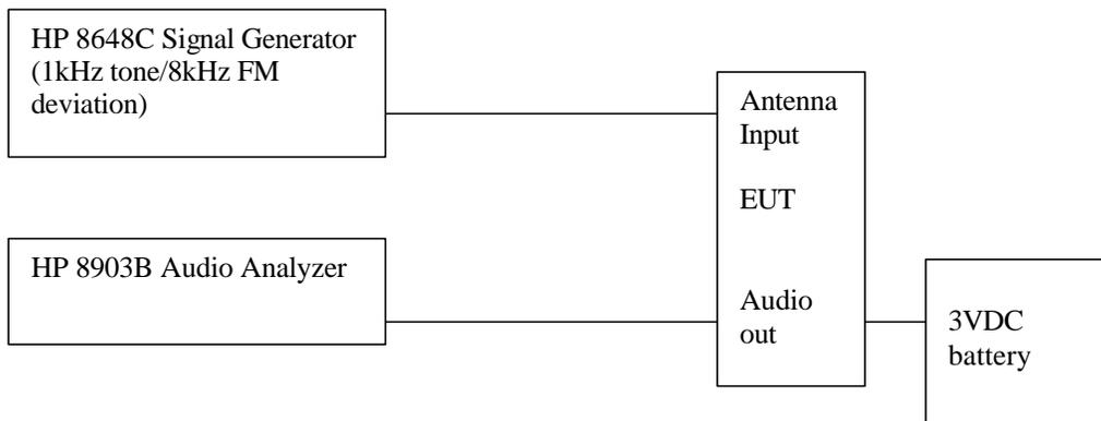
Frequencies used on the Signal Generator were 824.04, 836.50, 848.97 MHz for the Mobile and 869.04, 881.50, 893.97 MHz for the Base.
