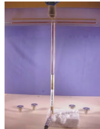
300MHz System Check Setup Photograph
