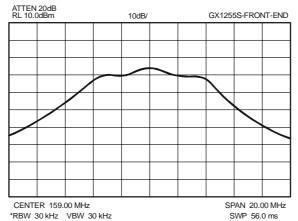
**Note**: Adjust the output of the tracking generator so that RF AMP and spectrum analyzer will not saturate.
