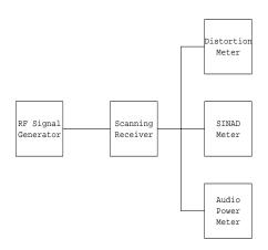
System Sensitivity measured in step 5 = 130 dBm
