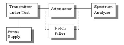
**METHOD OF MEASUREMENT:** The procedure used was ANSI/TIA 603-C:2004 without any exceptions. The measurements were made at TIMCO ENGINEERING INC. 849 N.W. State Road 45, Newberry, Florida 32669.
