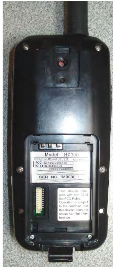
Back of DUT - Battery removed
