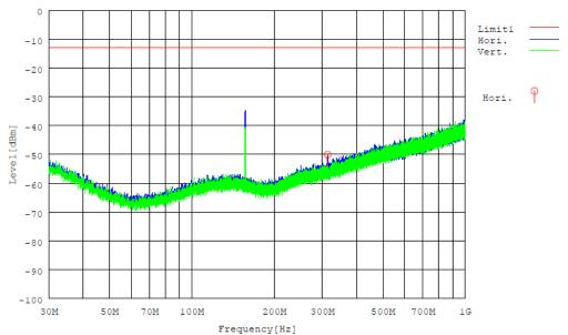
Note: 156.8 MHz is Tx carrier frequency.
