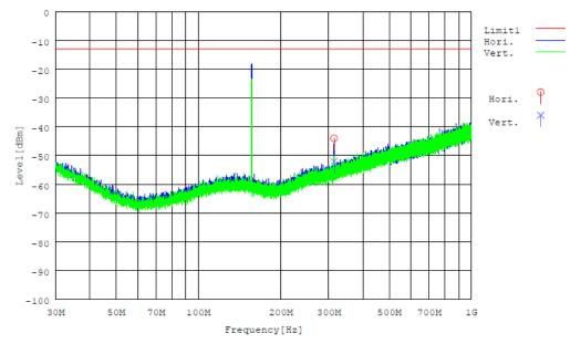
Note: 156.8 MHz is Tx carrier frequency.
